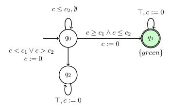
Figure 2.: A TBA  $\mathcal{A}$  that accepts the runs that satisfy formula  $\varphi = \lozenge_{[c_1,c_2]} \{green\}$ .
