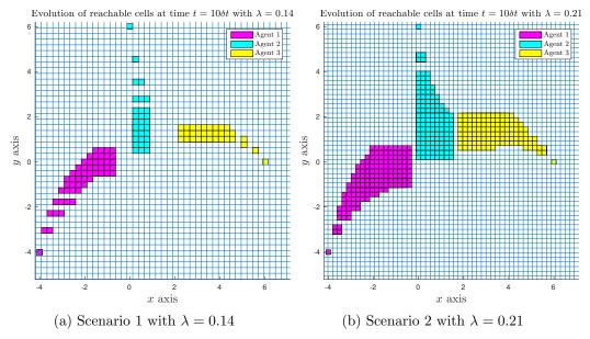
Figure 9.: Two simulation scenarios with N=3 agents and  $\lambda=0.14$ ,  $\bar{d}_{\rm max}=0.25$  (Figure 9a) and  $\lambda=0.21$ ,  $\bar{d}_{\rm max}=0.20$  (Figure 9b)) in a time horizon of  $t=10\delta t$ .
